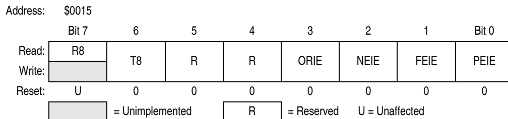
Figure 13-12. ESCI Control Register 3 (SCC3)
