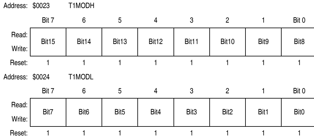
Figure 17-7. TIM1 Counter Modulo Registers (T1MODH:T1MODL)
